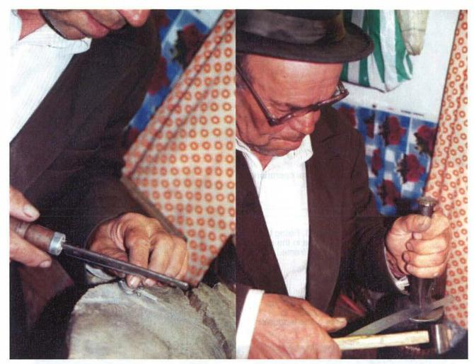
Fig. 11. Sawing the tongue's notch into the frame.
