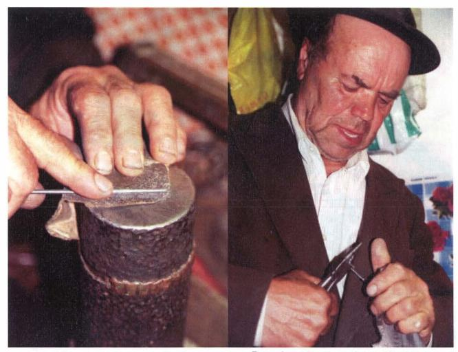
Fig. 7. Shaping the iron rod for the frame.
